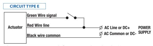
Valve actuator starting position can be factory set up on demand as either OPEN or CLOSED. If the valve is set-up in the open position the closing of the switch will drive it to the alternate position, and vice versa.
